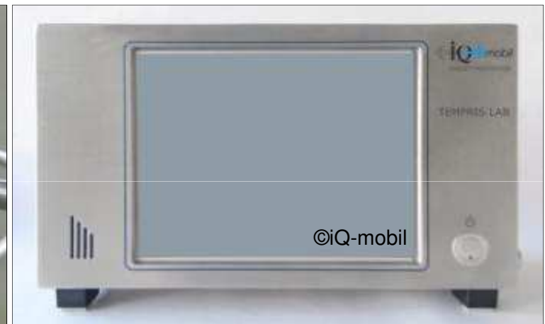
Interrogation Unit (IRU) with Computer
