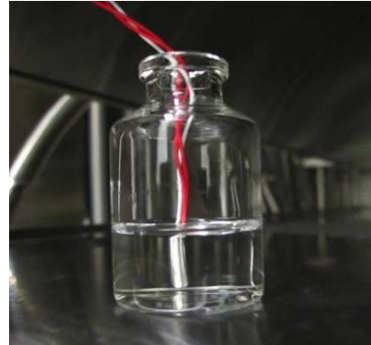
RDT - PT100 (positive temperature coefficient)
